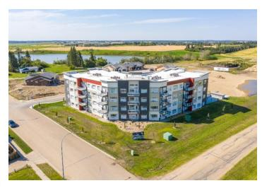
Eagle Builders, is a concrete - steel structure. That means it is fire resistant. There is very little that is combustible in this building. Also, our insurance bill is far less than it would be with a wood structure which means it is cost effective for you. The walls are a foot thick with 4 inches of concrete, 4 inches of solid Styrofoam insulation and another 4-inch slab of concrete. This 1-foot-thick wall makes up all the outside walls.
